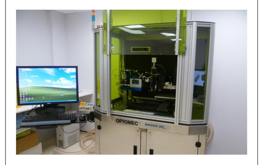
Aerosol Jet Deposition (AJD) is a digital process allowing designs to be rapidly created, modified, and printed whilst using small quantities of ink.
