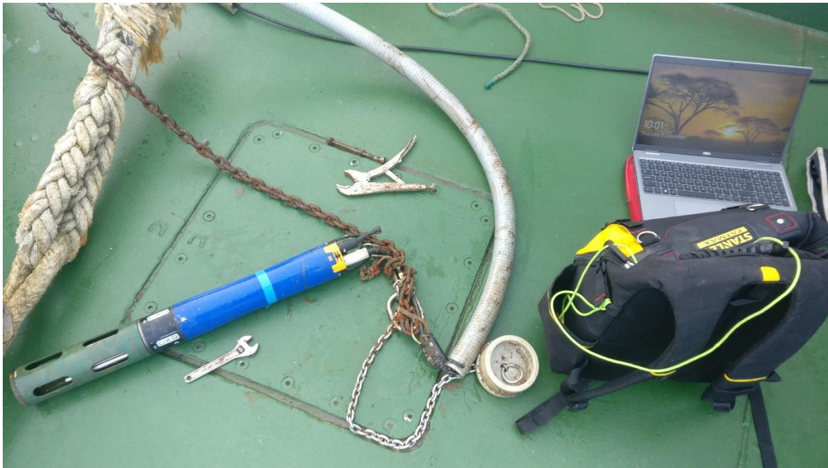
Figure 3 An Exo2 Sonde on the deck of the BIM barge in Castletownbere.
