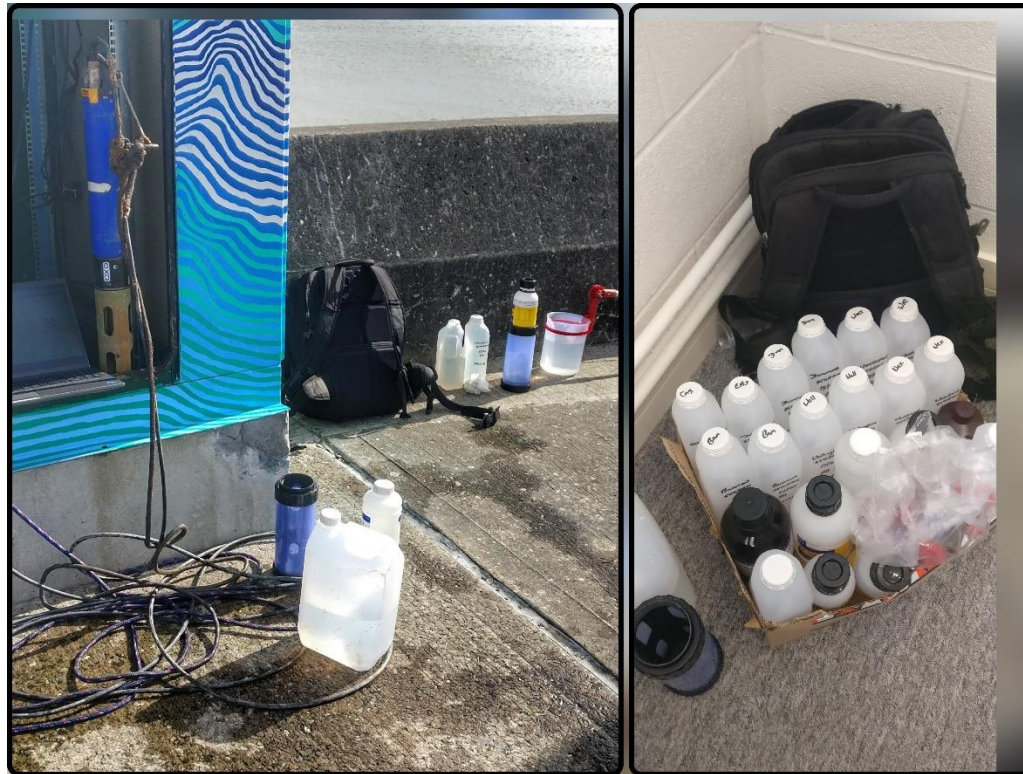
Figure 1. Exo2 Sonde, calibration solutions and sample bottles
