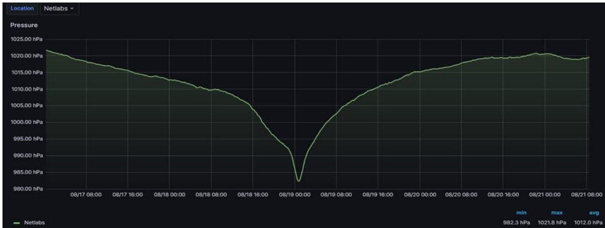
Figure 1. STREAM measurement of atmospheric air pressure in Waterford.
