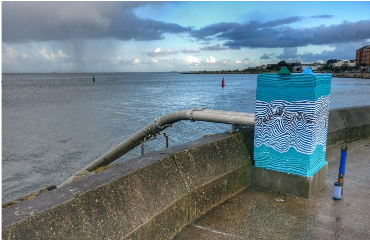
Figure 2 Wexford County Council sensor box housing STREAM water quality sensors.
