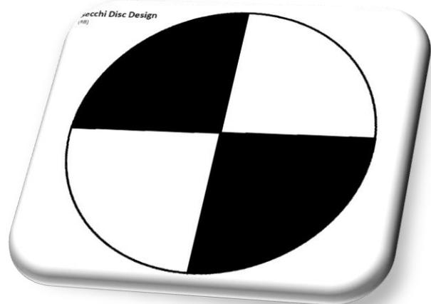
To measure the transparency of the water with a secchi disc, carefully lower the disc into the water while holding it steady with one hand and feeding a slack measured line with the other hand. Keep lowering the disc until the contrast (black and white) is no longer visible. Then, slightly raise the disc to see it again, and drop it slightly until it disappears again. Record the distance between the surface of the water and the disc.
