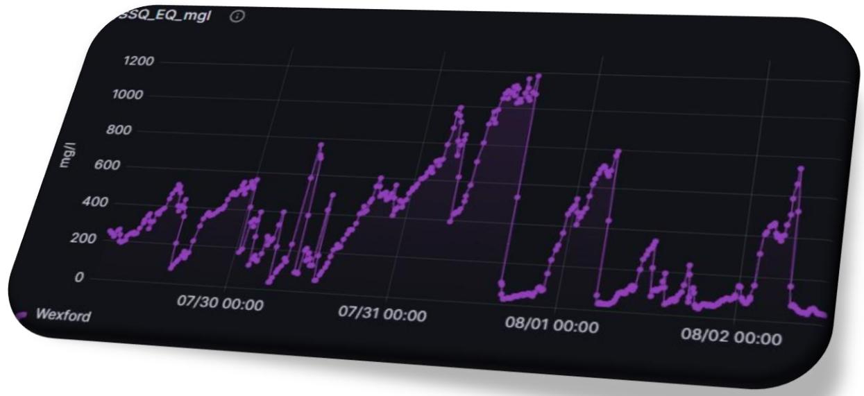
Turbidity is primarily attributed to total suspended solids (TSS), and the estimation of TSS levels using sensors has been calculated using linear regression modelling based on turbidity measurements. Parameters with the eq prefix are associated with the TriOS OPUS spectrometer, the company has developed a library of absorption spectra associated with the parameter.
