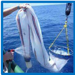
Figure #3: Washing down captured phytoplankton into the sample cup 2
