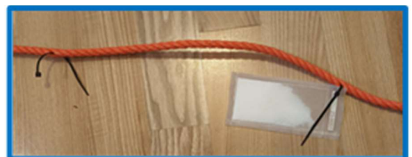
Figure #5: Redesigned SPATT bags with integrated 'numbered' laser-cut plastic label connected to deployment line.
