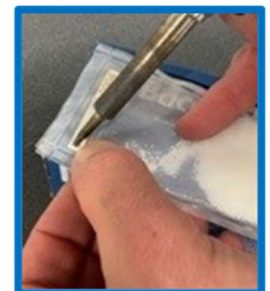
Figure #4: Application of a soldering iron to generate hole in label for zip tie attachment.
