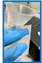
Figure #3: Filling SPATT bags with adsorbent phase, using funnel.
