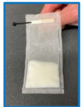
Figure #2: Redesigned SPATT bags with integrated ‘numbered’ laser-cut plastic label, with all four sides heat sealed.
